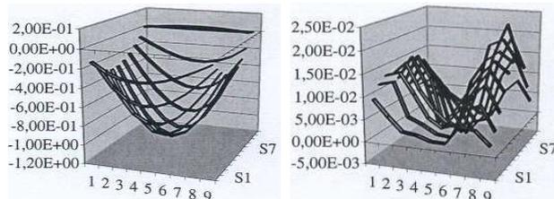
Fig. 8 Comparison of deflections of bridge girder for 11 time moments under mass 100 t travelling with two velocities: 36 and 3600 km/h (see Refs 44, 45, 56, 71). In the 11-th moment loading is after the bridge.
