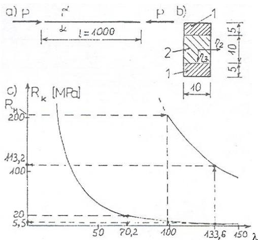
Fig. 4 Diagram of critical stresses in function slenderness  $\lambda$  for analysis of ultimate (global) slenderness for whole compressed bar composed from steel ((1) and timber (2) (see Ref.27)
