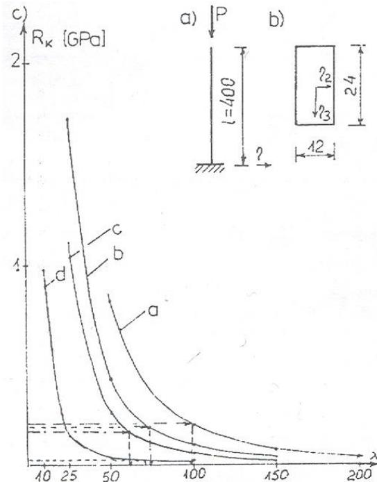
Fig. 3 Diagram of critical stresses in function of slenderness for homogenous bar, made from some different materials: a) steel, b) brazen c) aluminium, d) timber (see Ref. 27)
