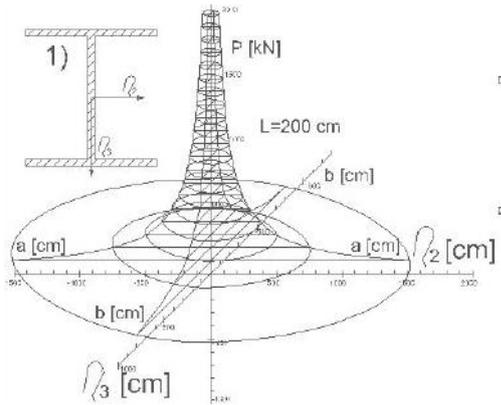
Fig. 6 Ultimate critical iso-surface for the compressed straight bar with I cross-section and with length  $L=200$  cm, (see Ref. 68, 69). The diagram indicates critical force position and its value.
