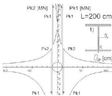
Fig. 7 Diagrams of critical forces  $P_{k1}$ ,  $P_{k2}$ , and  $P_{k3}=P_2$ . The last is much bigger from critical force  $P_{k1}=P_{k2}$ . The bar has the length  $L=200$  cm and I cross-section (see Refs 68, 69). The bar is compressed eccentricly by force located on vertical axis of symmetry
